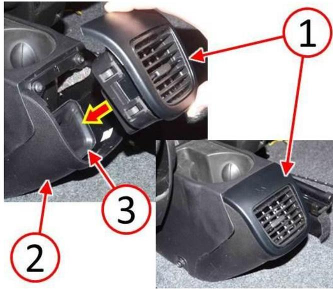
**Fig. 12 Install Floor Console Air Outlet**
