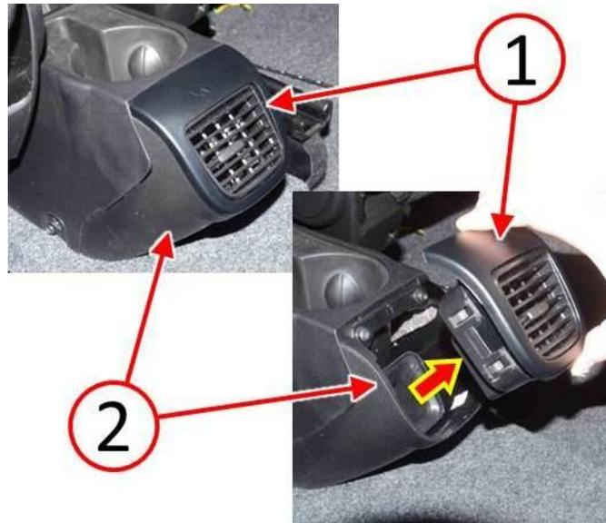
**Fig. 1 Remove Floor Console Air Outlet**
