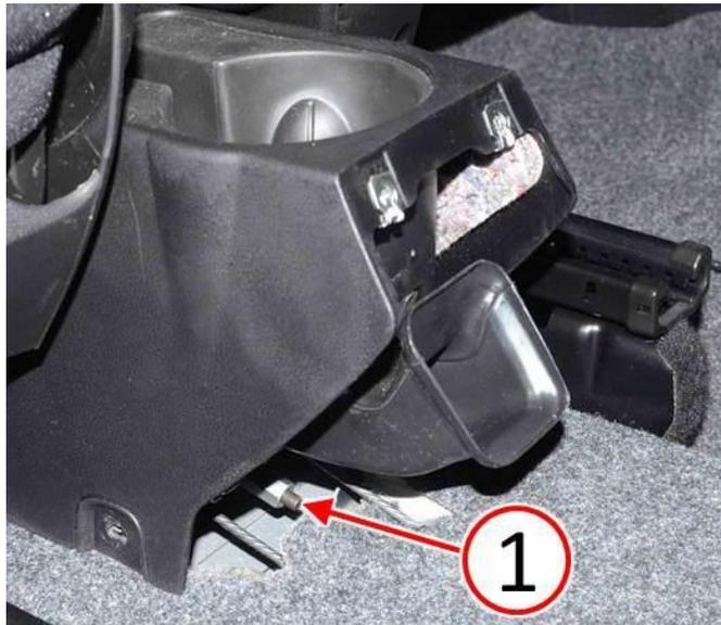
**Fig. 10 Adjust Parking Brake Cable**
