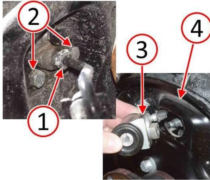
**Fig. 6 Replace Rear Wheel Cylinders**
