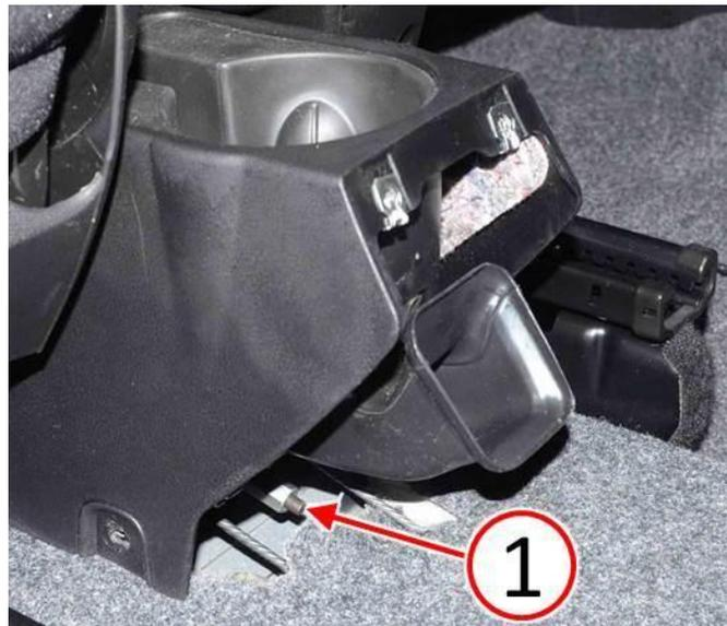
**Fig. 3 Loosen Parking Brake Cable**
