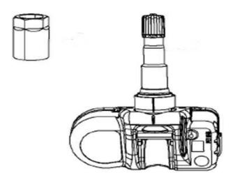
Fig. 2 Steel Valve Stem
