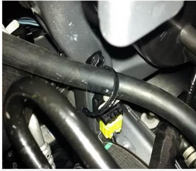
Fig. 1 Location Of The Tie Strap
