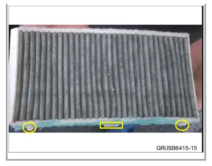
6. Allow the applied glue time to dry then then install the upper and lower micro-filters in the housing (REP 64 31 010).
