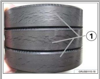
Surface cracks (1) form on the drive pulley over time.
