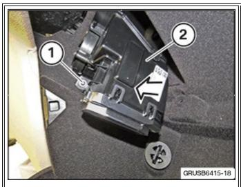
Correctly position the new air freshener (2) and press firmly until the latches engage.
