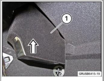
Correctly position the air freshener cover (1) and press firmly in the direction of the arrow until the latches engage.
