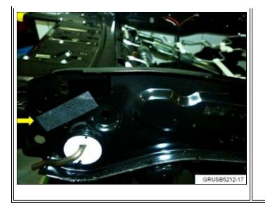
the front metal area as shown. Note: The seat cover and plastic bracket were removed for illustration purposes only, and show the location of the felt to be applied. After the felt tape is applied, rivet the bracket to the seat frame. Install all removed parts in the reverse order of their removal, and then quality check the repair.
