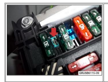
3. Check Fuse 203 fuse slot and if there are any signs of overheating, replace the rear power distribution box. Refer to ISTA repair manual "61 13 042 Replace power distribution box (luggage compartment)".
