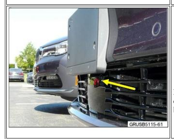
4. The approved bracket installation must look like the picture. This will provide the needed clearance for the ACC sensor (yellow arrow).
