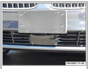
Note: The bracket is included with vehicle from factory (uninstalled).
