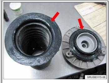
Apply a thin coat of lubricating grease P/N 07 55 9 056 992 or P/N 83 23 0 301 796 to the entire surface of the spring pad and spring strut support bearing
