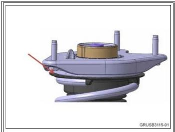
Lubricate the surface between the spring pad and spring strut support bearing. To do this, the support bearing must be removed. Refer to ISTA REP 3133001 "Replacing the spring strut support bearing at the front left or right".
