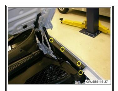
1. Remove the sealing trim from the left-hand side panel
