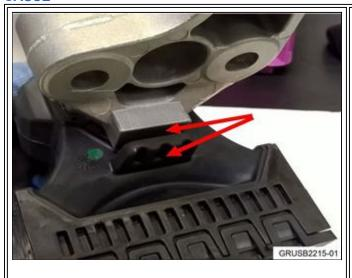
Friction between the engine mount and its contact surface with the rear axle.
