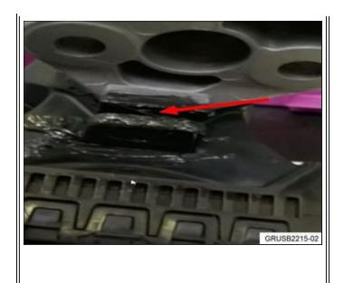
3. Apply grease (P/N 07 55 9 056 992) to the contact point between the engine mount and right rear axle.
