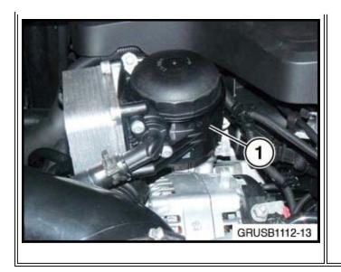
3. If the vehicle is fitted with the plastic engine oil filter housing (black color) then replace the engine oil filter housing as per the attached instructions.
