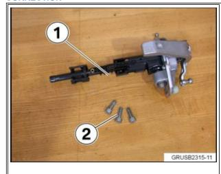
The shifter tower for the transmission will need to be replaced. The repair kit (P/N 23 00 8 654 531) consists of the improved shift tower and three screws. A flange gasket sealer (P/N 83 1 90 422 969) will also be needed to complete the repair.
