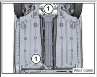
If work was performed on the vehicle which made it necessary to loosen the M10 x 40 mm screw connections between the HV battery and front/rear axle carries (1), follow the procedure steps below.
