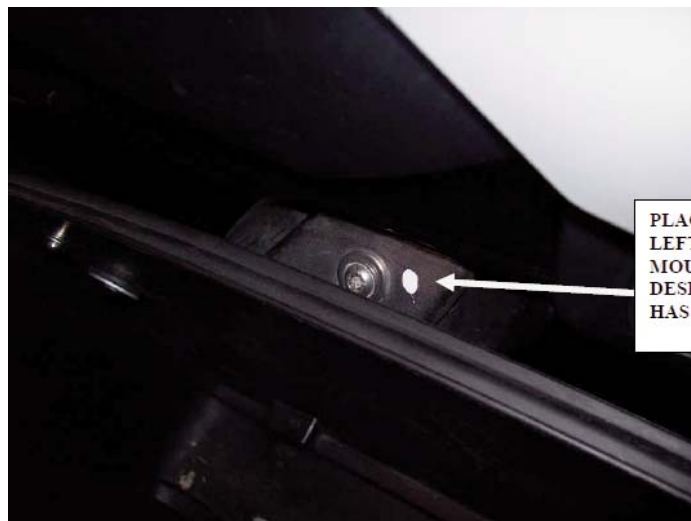
Rubber Insulator installed with wire tie. Installed under Harness between "T" Bracket.
