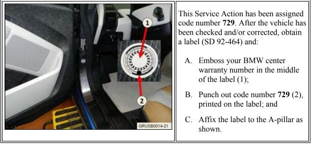
If the vehicle already has a label from a previous Service Action/Recall Campaign, affix the new label next to the old one. Do not affix one label on top of another one because a number from an underlying label could appear in the punched-out hole of the new label.
