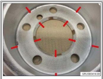
Sand the hub surface on the **brake disc** to the wheel bearing hub using 80-grit sandpaper.
