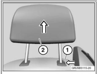
Press the latch mechanism (1) and lift out the head rest (2) in the upward direction.
