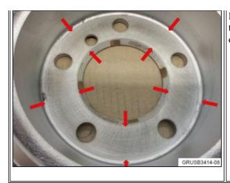
Do not apply any type of lubricant to the components surface (wheel bearing or brake disc).
