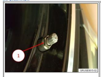
The valve stems are single-use only, and must be replaced every time the RDC/RDCi wheel electronics are replaced.
