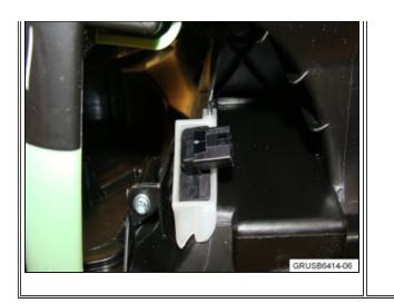
Ensure the evaporator temperature sensor is correctly seated.
