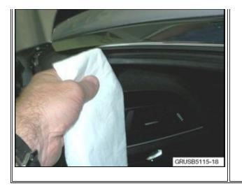
3. Use a clean lint-free cloth to remove the excess lubricant. Continue buffing until the seal surface no longer has a glossy finish.
