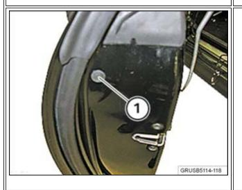
2. To remove the driver's exterior door handle, pry out the cover cap (1) and remove the screw underneath.
