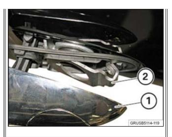
3. Partially pull out the exterior door handle (1). Feed out the retaining plate (2).
