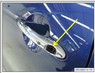
1. The driver's side exterior door handle cover cap is loose or missing.
