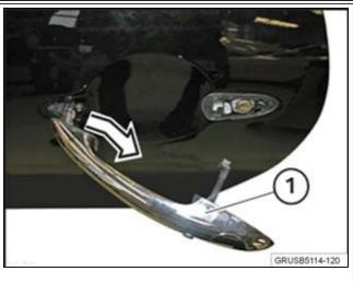
4. Pull the exterior door handle further (1) towards the rear. Feed out the handle from the door. If necessary, unlock the associated plug connections and disconnect; then remove the exterior door handle.
