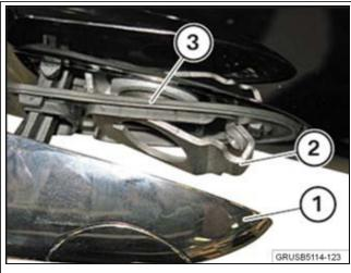
7. Position the exterior door handle slightly outward (1). Feed in the retaining plate (2). Ensure the gasket (3) is seated correctly.
