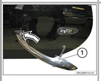
5. To install the driver's exterior door handle, first connect the plug connections; then feed the exterior door handle into the front opening.
