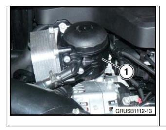
engine oil filter housing as per the attached instructions.
