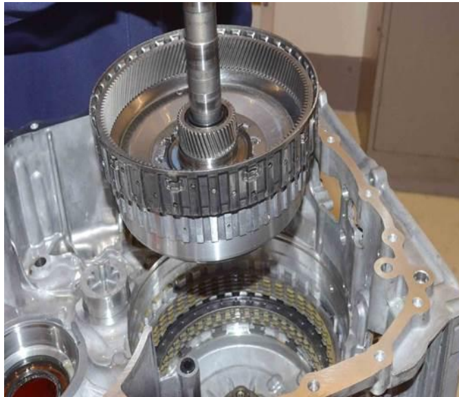
Fig. 9 Gear Train Assembly
