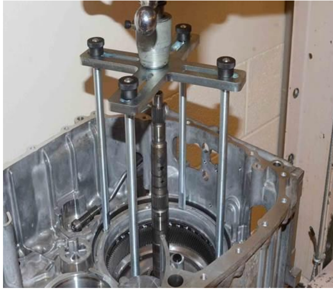
Fig. 8 Pressing Tool Installed
