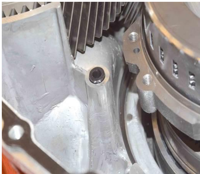
Fig. 21 Transmission Fluid Port Seal
