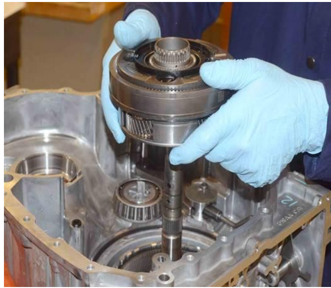
Fig. 6 Gear 4 Planetary Pinion Carrier Assembly
