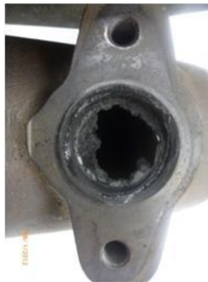
Figure 2 – Partially plugged AFI port
