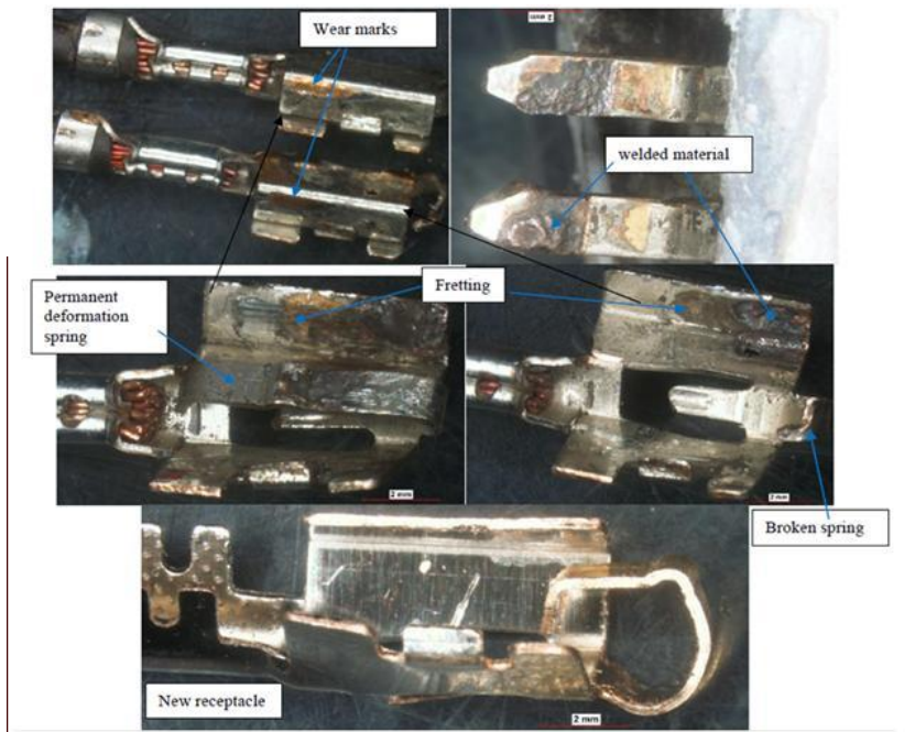
Figure 6: Examples of damage to the IPR valve pins and connector
