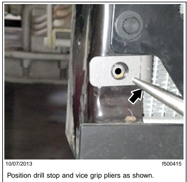
Fig. 4, Drill Stop Installation
