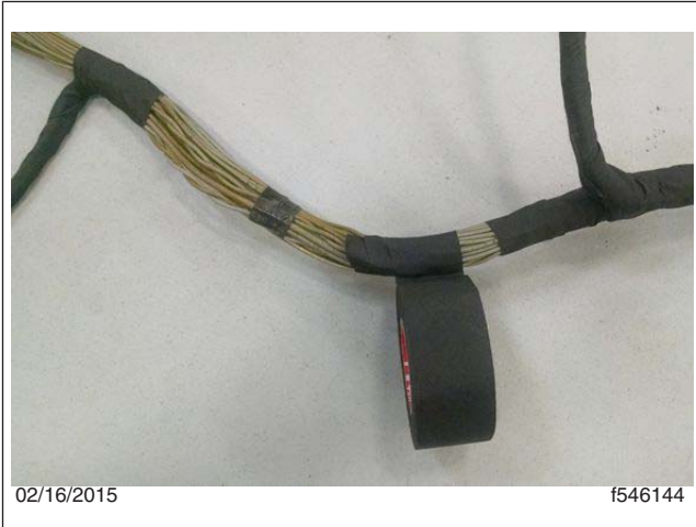
Fig. 14, Wrapping the Harness with Fiber Tape
