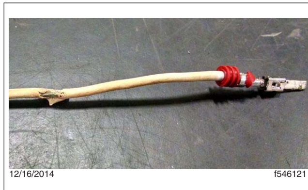
Fig. 2, Insulation Discoloration, Major
