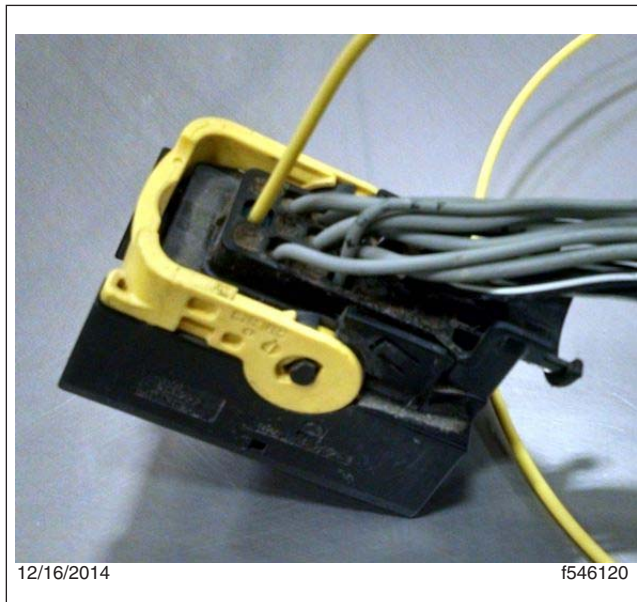
Fig. 3, Terminal Inserted Into the Connector
