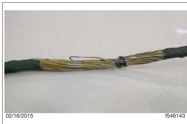
Fig. 12, Overlay Added to the Damaged Area of the Harness
