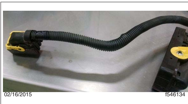
Fig. 7, Harness Wrapped with Convolute
