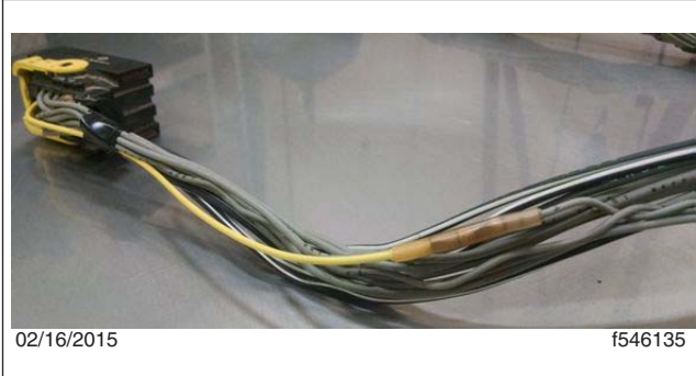
Fig. 5, Splicing the Wires
