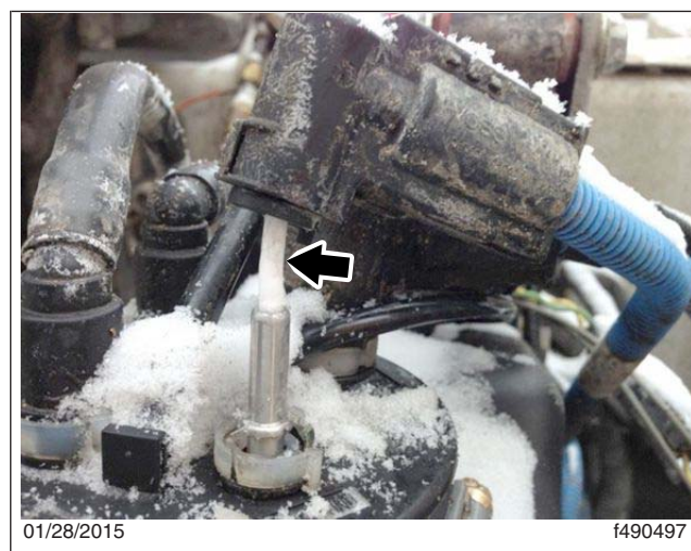
Fig. 1, Ice Expansion at the DEF Line Fitting
