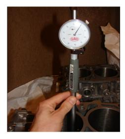
A Dial Bore gauge is the easiest and quickest way to measure cylinder bores accurately although significantly more expensive to purchase than a set of "T" gauges.
