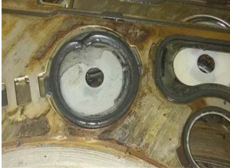
Figure 2 Example of a failed cooling passage grommet on the cylinder head gasket
