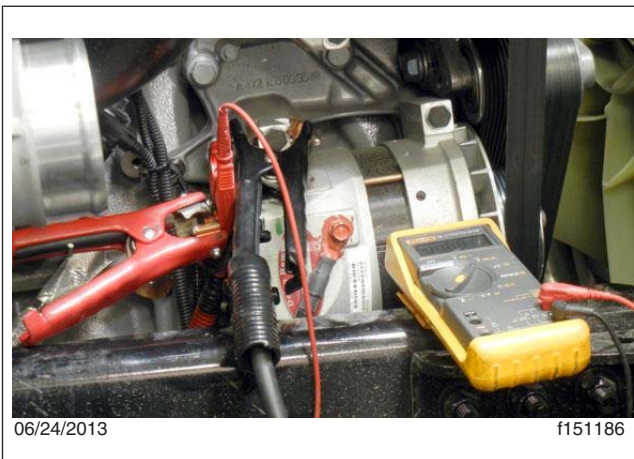
Fig. 5, Alternator Positive Cable Check
