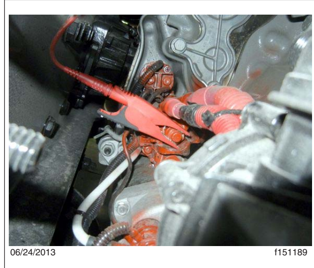
Fig. 8, Location of the starter positive post.
