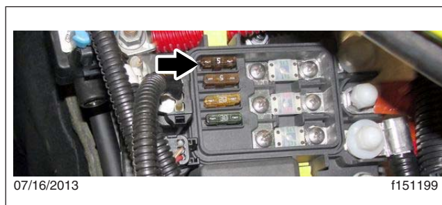
Fig. 15, EPA10 vehicles: 5 amp remote sense fuse, location D in the Powernet Distribution Box (PNDB).
