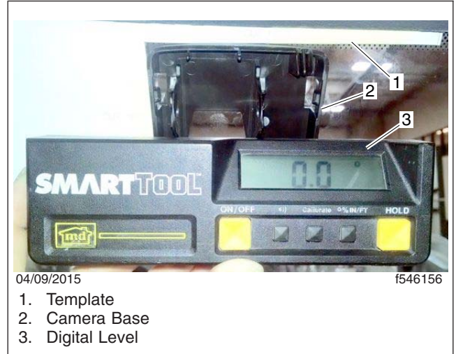
Fig. 8, Aligning the Base with a Digital Level
