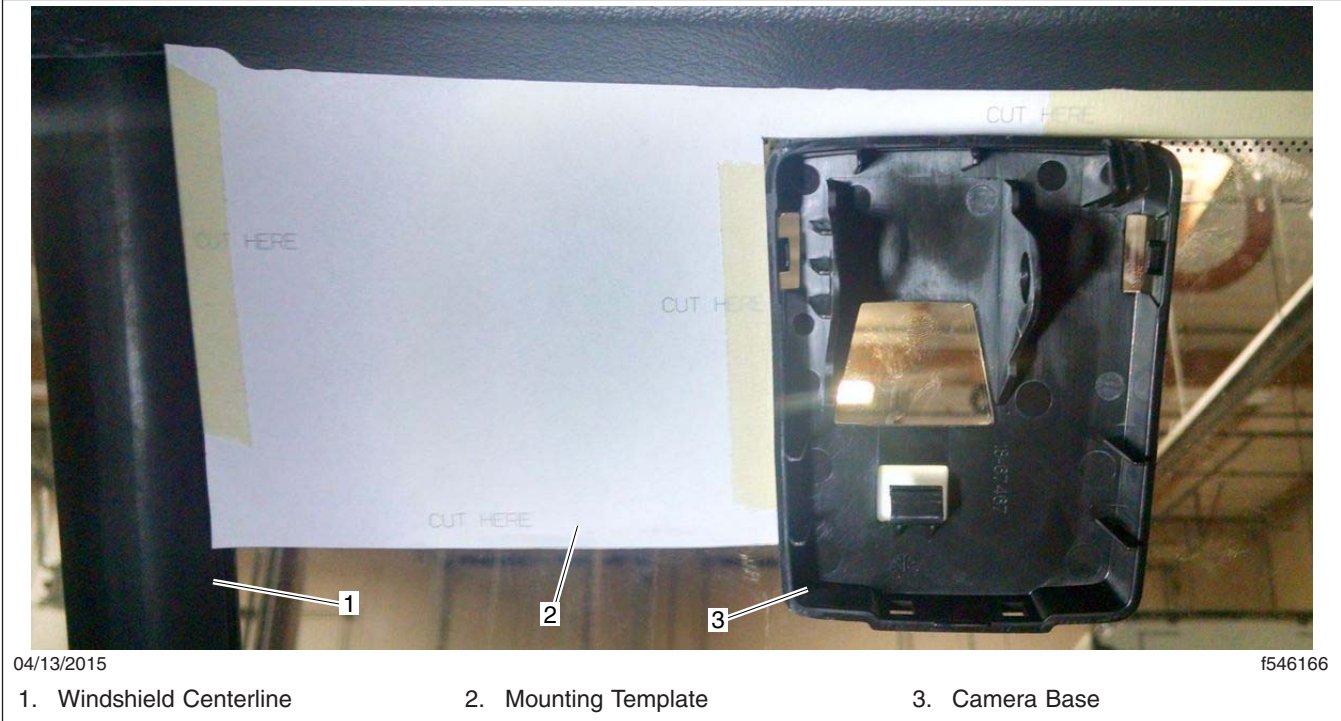
Fig. 6, Mounting the Camera Base using the Template
