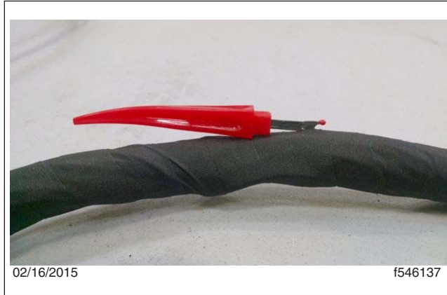
Fig. 9, Cutting an Opening into the Fiber Wrap
