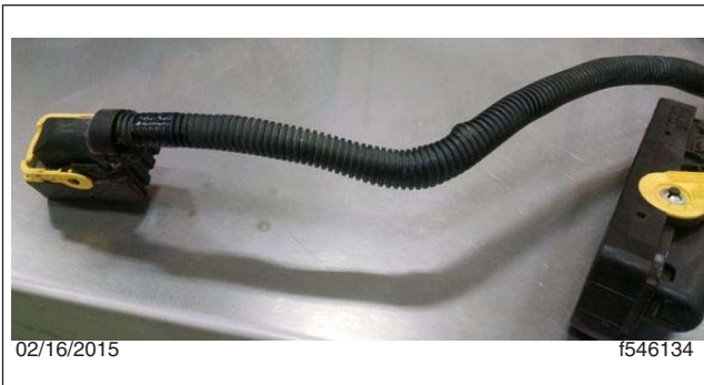
Fig. 7, Harness Wrapped with Convolute
