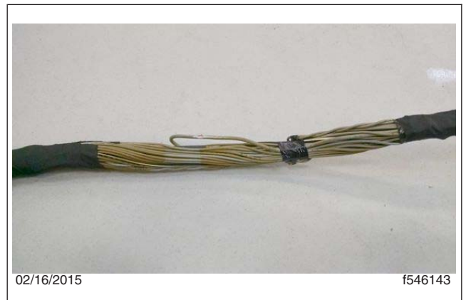
Fig. 12, Overlay Added to the Damaged Area of the Harness
