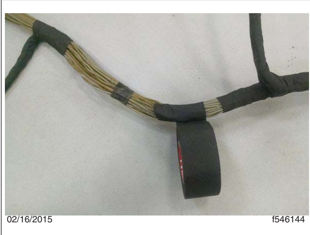
Fig. 14, Wrapping the Harness with Fiber Tape
