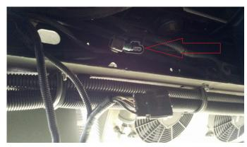
1. Disconnect the LPG fuel pump connector X350.
