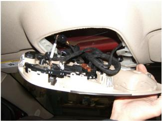
1. Remove the Mobile Telephone Microphone. Refer to Mobile Telephone Microphone Replacement in SI.
