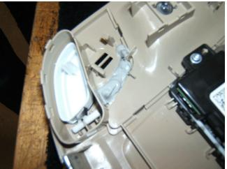
3. Using engine sealant, evenly apply to the area shown being careful not to get any sealant onto the microphone grille opening. Spread the sealant evenly
