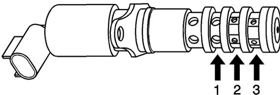
(1) Screen for Advance Pressure to Camshaft Actuator
