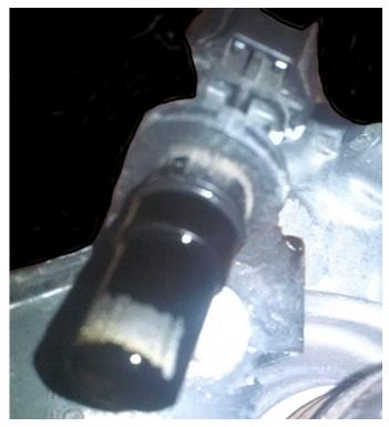
If an excessive amount of debris in found on any one of the speed sensors remove the transmission fluid pan.
