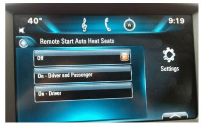
However, this is actually an Off / On system – meaning it's either both seats off or both seats on during a remote vehicle start event. The menu option the customer should see is an Off or On selection, as shown below.
