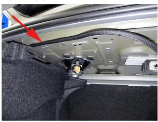
Install a protective cover (sealing strip) on the edge of the rear window panel as shown.
