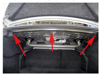
Ensure the sealing strip covers the complete edge between the left and right trunk side panel trim.
