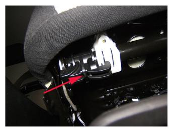
4. Install a nylon wire tie as shown. Trim the excess wire tie material.
