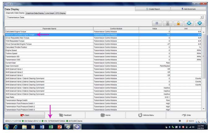
Notice: This is a typical GDS 2 "individual" screen shot taken from a Model Year 2015 Sierra showing the: VIN and Maximum Calculated Engine Torque Parameter
