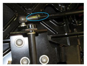
2. To aid in determining the **one revolution** of adjustment, mark the original position of the driver's side jamb nut and ball socket.
