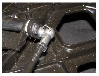
**Note:** The above graphic shows the locking retainer in intermittent position for illustration purposes only. When fully installed, the retainer is rotated and snapped tightly around the link rod.
