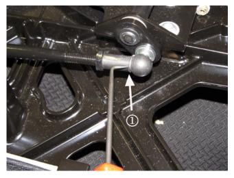
**Note:** When removing the link rod from the latch, you must remove the locking retainer (1), make the rod adjustment, then be sure to reinstall the retainer.
