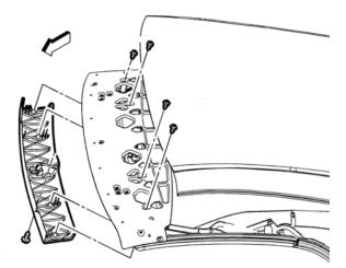
1. Remove the folding top #1 bow garnish molding. Refer to Folding Top Number 1 Bow Garnish Molding Replacement in SI.
