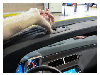
2. Using your little finger (as shown in the graphic above), reach in the driver's side latch striker and toggle the micro switch while observing the DIC. The "Top Not Secure" message should also toggle off and on.
