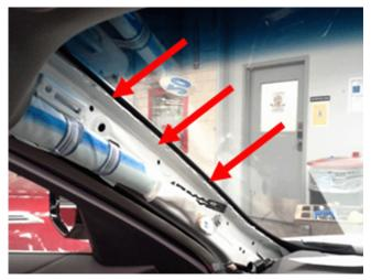
7. Re-water test the repaired side(s) and inspect for any water visible at the interior A-pillar.
