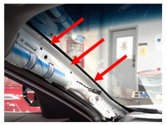
4. Continue to flood the area for up to five minutes, while having an assistant sit inside the vehicle observing the interior A-pillar for any evidence of water running along the pillar.
