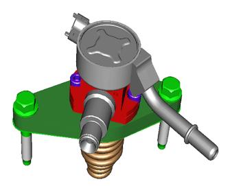
Delphi style fuel pump part number 12673522 and fuel pipe part number 12673079 as shown above.
