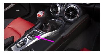
Driver Mode Control Switch: The Driver Mode Control has three or four modes: Tour, Sport, Snow/Ice, and Track. The Track Mode is for V8 models
