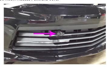
The tow hook (shown installed) access **point** on the Camaro was uniquely packaged in the front grille to keep a clean, bold, front end appearance. The LT and the GM accessory grille do not have a tow hook access **cover**. To access the tow hook access **point** on the SS, a small **cover** will need to be removed.
