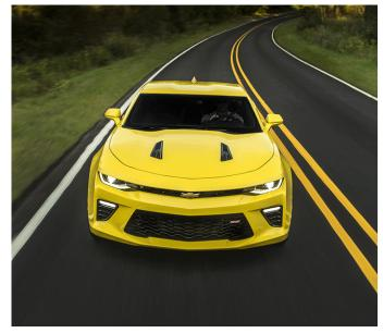
The SS hood has functional air vents that help to improve engine cooling and reduce front end lift, while the SS front fascia has integrated brake cooling ducts. Standard HID headlamps on the SS are available on the LT with the RS Appearance Package. LED daytime running lamps are standard on all models.
