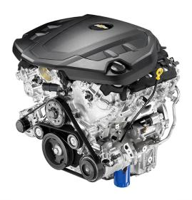
For 2016, the all-new V6 3.6L — RPO LGX is standard in the Camaro LT versions. The LT can be equipped with the 8-speed 8L45 automatic transmission — RPO M5T or the Manual 6-Speed Tremec — RPO M13. The engine produces an SAE certified 335 horsepower (250 kW) at 6,800 rpm and 284 lb-ft (385 Nm) of torque at 5,300 rpm.
